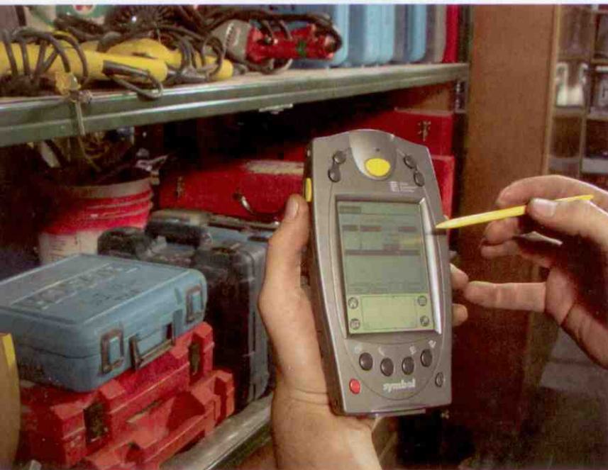
Computerized systems, such as this QuickPen scanner, provide a detailed history of all tool movements.
